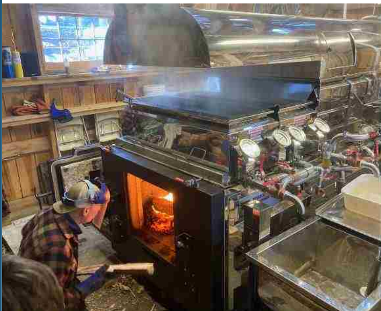
Lamb Sugarworks’ partner Jim Olmsted seen loading wood into the evaporator. Maintained at between 600 and 700 degrees Fahrenheit, in one season the evaporator will boil down as much as 60,000 gallons of sap to produce over 1,000 gallons of maple syrup.
