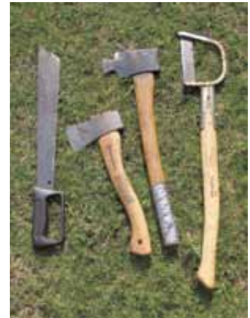
Cutting tools for hack-and-squirt treatment.
